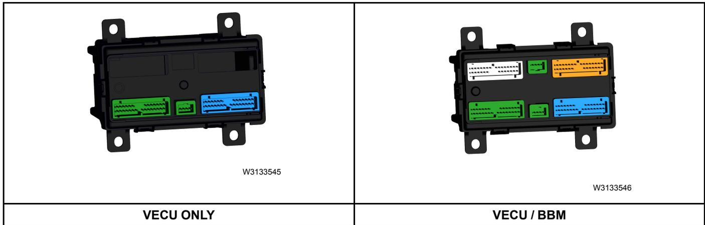
**Note:** BBM will have the white and orange connector plug and the VECU will have the blue and green connector.
