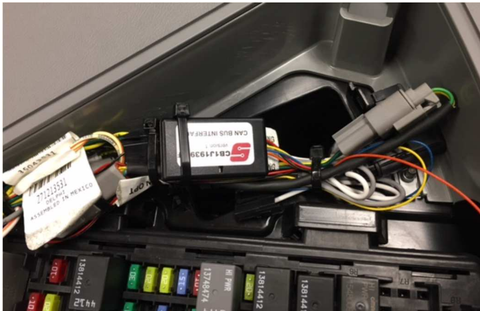
Fig. 45 CAN Bus reader installed
